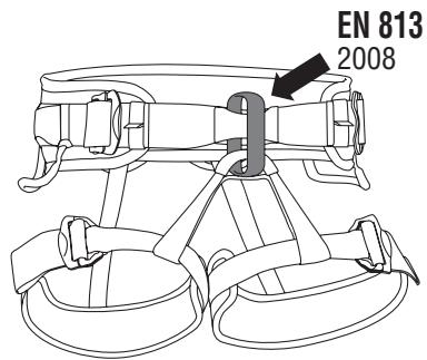
Ventral attachment point made up of two textile bridges or the connection ring.
