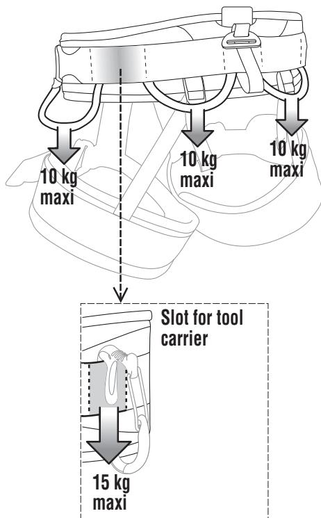
The equipment loops must only be used to attach and support equipment.
